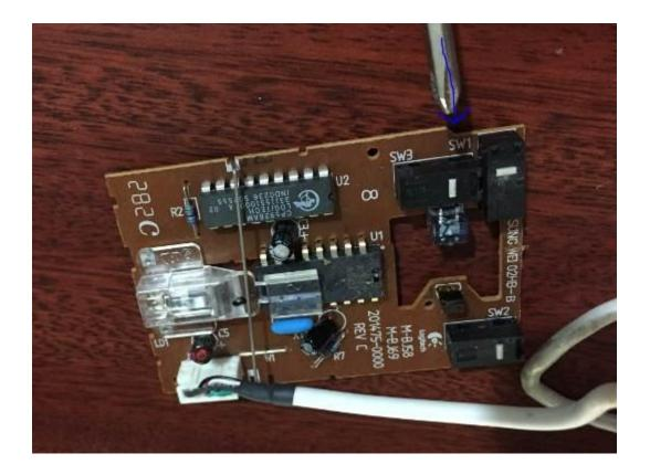
Connect the USB mouse cable to identify the correct switch (if required). Press the button to activate any computer icon
